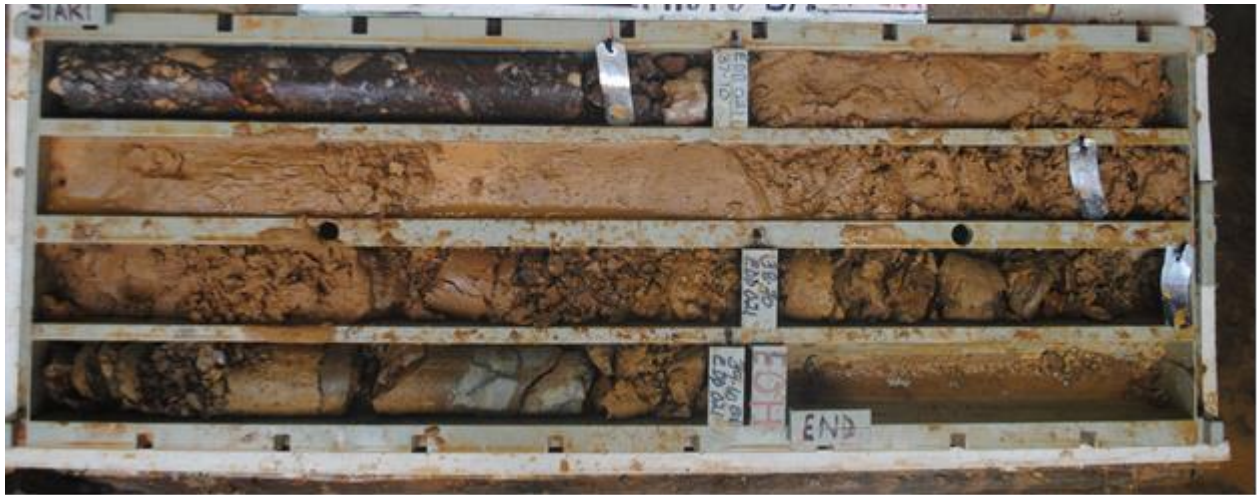
Picture of partially leached oxidized Quartz mangano-carbonate limonite vein in hole EDD 021 from 35m to 37.10m depth interval.
